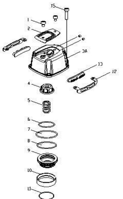
**ICB No. 98204 (CRN4500K4) Trigger Valve Assembly with Trigger Kit contains:**
